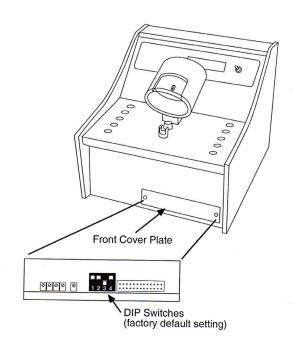
Simply raise dip switch 3 and replace the front panel of the Sonoclot Analyzer, if needed.
